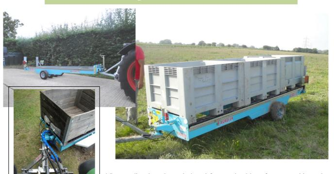
Larger model trailer showing drawbar turning angle
