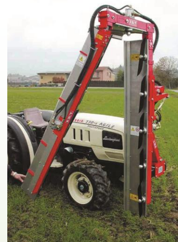
One of the vertical bars is fitted with a spring to avoid obstacles.
