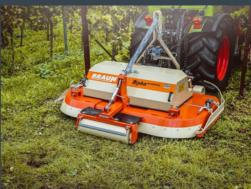
The 5mm-thick ball bearing stabilising wheels mounted on the base frame guarantee superior stability. Integrated implement support brackets of 50 x 50 mm for other accessories (such as vine stem cleaner etc) allow for additional work procedures to be performed simultaneously. Even vine prunings can be mulched thanks to the sturdy construction of the Alpha 2000.
