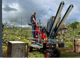
It even has an onboard computer, the M-Connect harvest registration system, which automatically records key harvest data allowing growers to track and trace fruit from the tree to the cold store.
